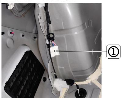
Factory connector for connection of the main plug WH1R cable-harness.
