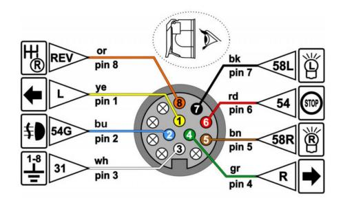
List of pins and colors pin 1 (ye) yellow pin 2 (bu) blue pin 3 (wh) white pin 4 (gr) green pin 5 (bn) brown pin 6 (rd) red pin 7 (bk) black pin 8 (or) orange
