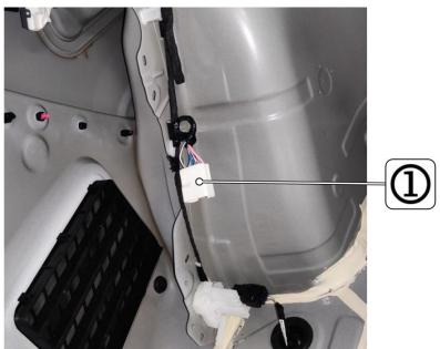
Factory connector for connection of the main plug WH3 cable-harness.
